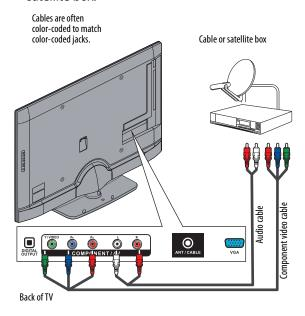
Connect an audio cable (not provided) to the L and R audio jacks on the back of your TV and to the audio out jacks on the cable or satellite TV box.
